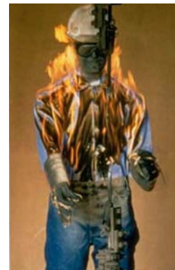
After Electric Arc Blast
