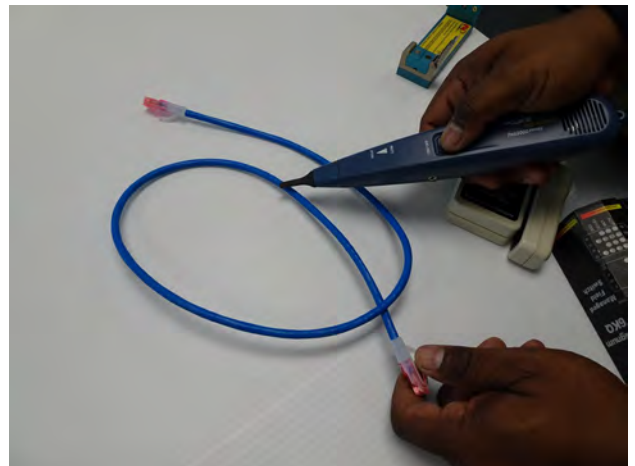
Figure 86 Fox and Hound Tool in Use - courtesy of MD MTA
