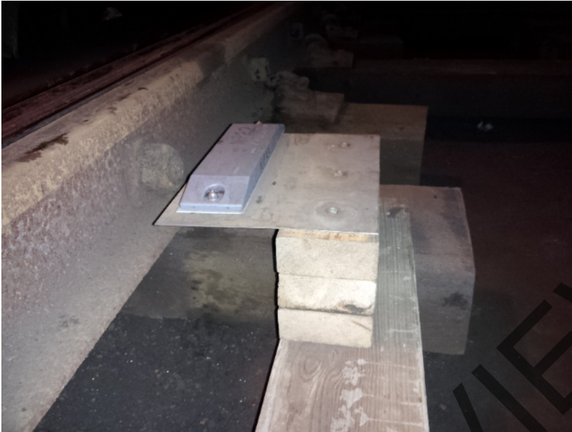
Figure 3.1 Norming Point with New Mount as to Minimize Space Between Reader and Norming Point - Courtesy SEPTA
