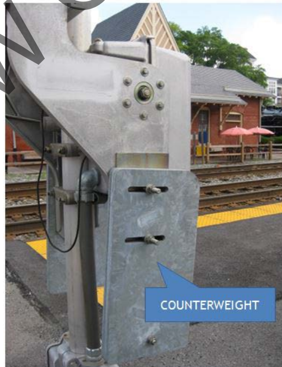
Figure 18 Gate Arm Counterweight
