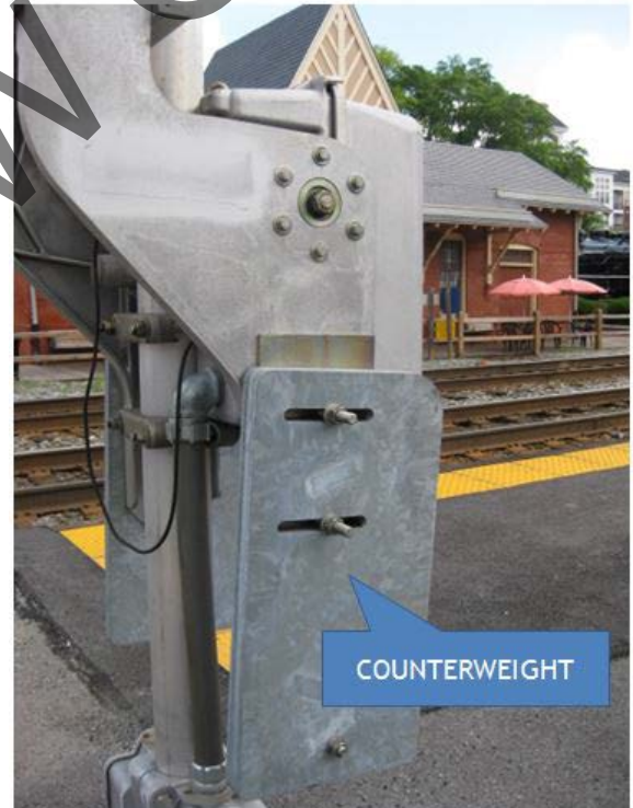
Figure 18 Gate Arm Counterweight
