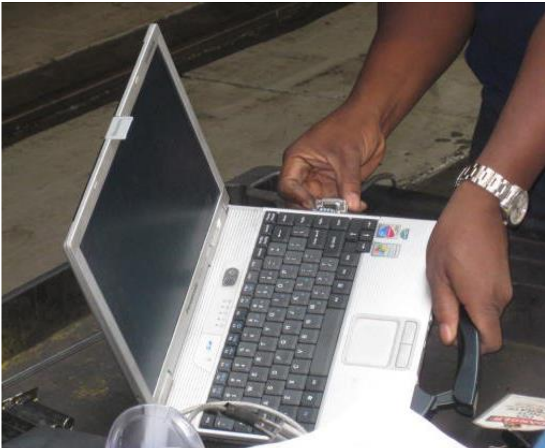
Figure 1.1 Rail Car Technician Connecting a PTU to the Bus of a Rail Vehicle, Courtesy of TLC
