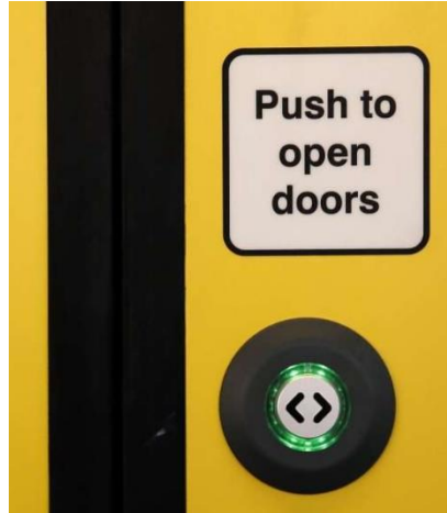
Figure 2.20 Example of a Rail Car Specific Switch
