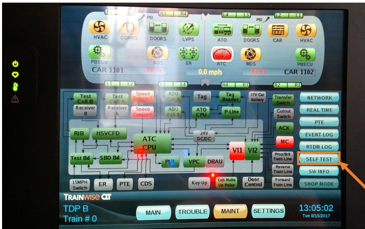
Figure 3.25 Accessing Self-Test Through the TDP. Courtesy of PATCO
