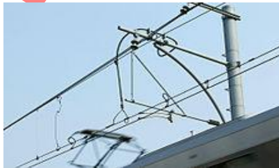
Figure 5 Overhead Catenary system
