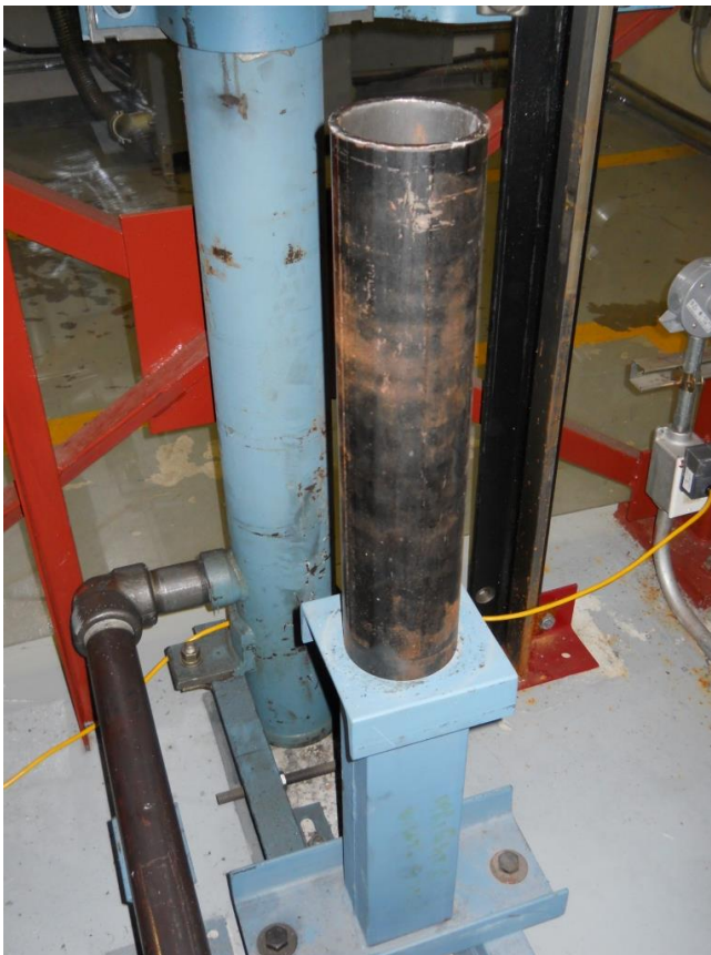
Figure 1.12 Placing the pipes on the buffer stand –Courtesy WMATA
