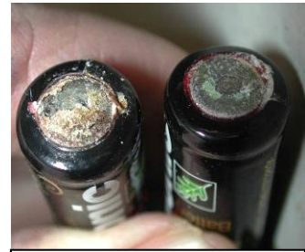
Corrosion on Batteries
