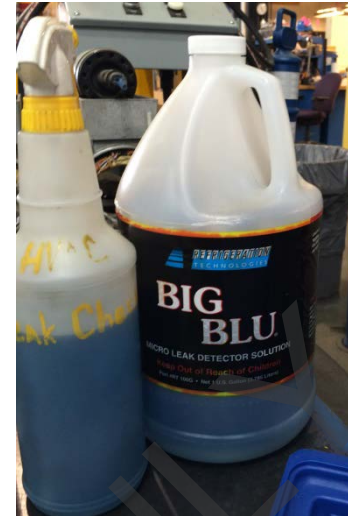
Figure 3.13 Big Blu Leak Detection Solution (Courtesy of CATS)
