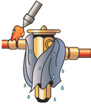
Figure 2.27 Wet Rag Wrapped Around TXV to Avoid Overheating
