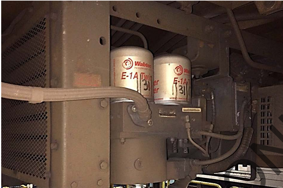
Figure 2.11 Air Compressor Unit on HRV –courtesy Maryland MTA
